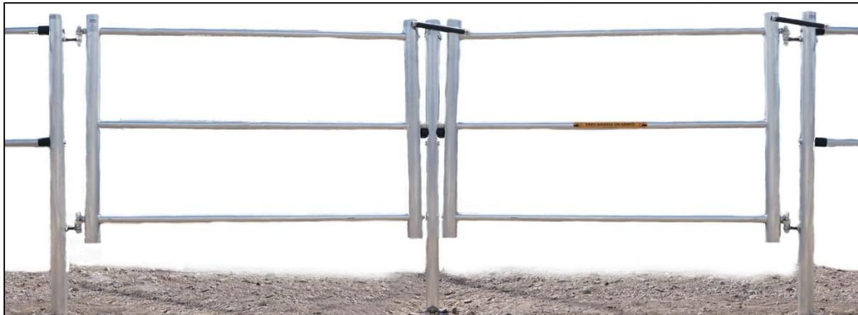
When installing four meter wide leaf gate the space must be left 4,38m. One vertical post in the middle will support the gates (1). A short spiral post must be installed for the vertical post to the ground(2). The end part of the short post is to prevent the post from rotating in the soil. The vertical post is screwed to the short post.
